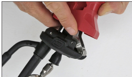
5: It should be fitting flush with the plastic surface on each side. It should not interfere with the release handle.
