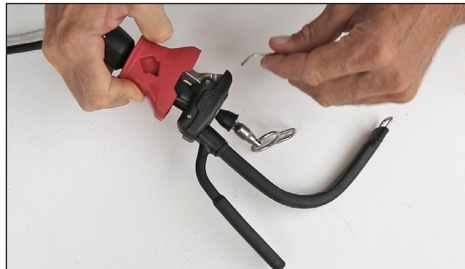
1: While holding the release handle up, use the 2mm Hex key to unwind the Hex screw that is securing the Stainless Steel Release Lever in place.
